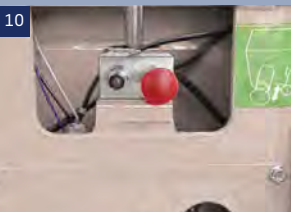
Manual release valve: When the machine can not move, you can push the machine after pressing this valve
